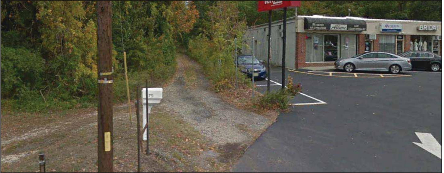
Image 1: Entrance to Highland Place off Highway 35. Approximately 14'-0" wide dirt road with acute angle entrance. Appear vehicles accessing Highland Place are illegally cutting across the exit drive aisle for the strip retail center.
